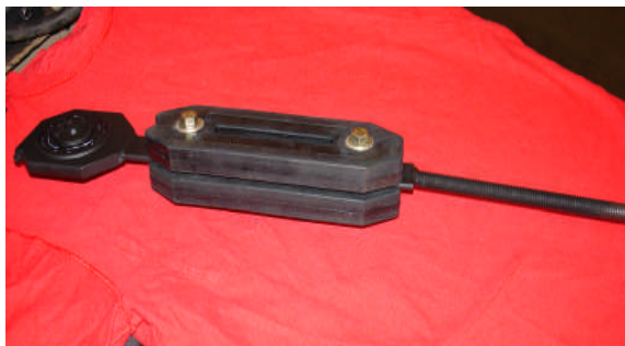
Main Shaft Clutch Assembly Eliminates Vibration
