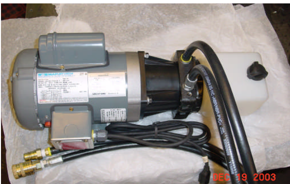
3/4 HP Farm Duty Motor and Direct Drive Pump
